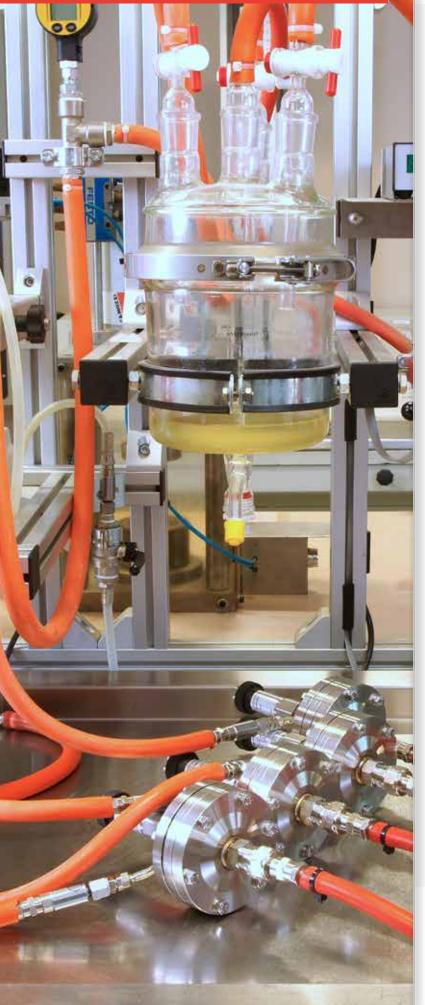
Design and manufacturing of diaphragm seals on specific customer request, also in special materials (Hastelloy, Monel, Tantalum..). Diaphragm seal mounting also on customers' instruments
